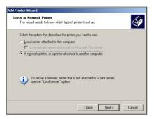
6. In the next window, select "Connect to a printer on the Internet or on a home or office network" by clicking in the appropriate circle, then enter the URL of the Print Server and printer in the "URL" text box. The format of the URL is as follows: http://Print Server IP address:631/printer port number. In the example below, the Print Server IP address is "192.168.2.1," and the printer port number (the Print Server port to which the printer is connected) is "p1." Click Next.
